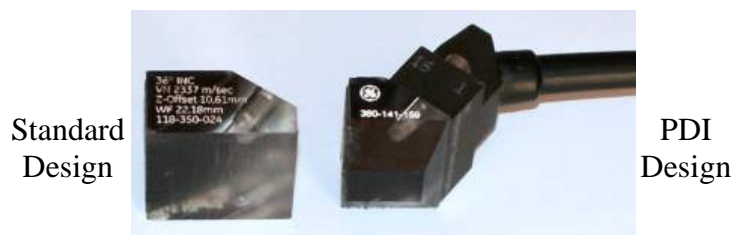
Figure 4. Standard Wedge versus PDI Wedge
