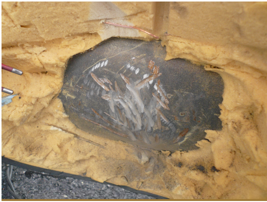
Figure 16: defect D2 (right): width 80 mm, length 92 mm, reduced area 5,8%
