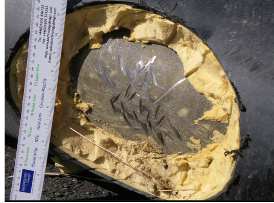
Figure 16: defect D2 (right): width 80 mm, length 92 mm, reduced area 5,8%
