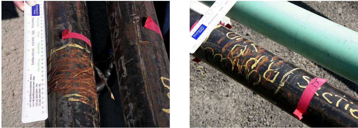
Figure 8: random grinded defects on sample 3
