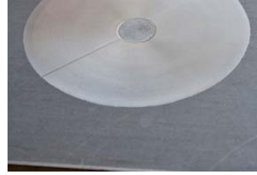
Figure 13: Artificial flaw simulating the decrease in wall thickness due to corrosion.
