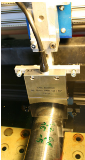
Figure 3: Round-bar testing with curved linear arrays [7] [8]
