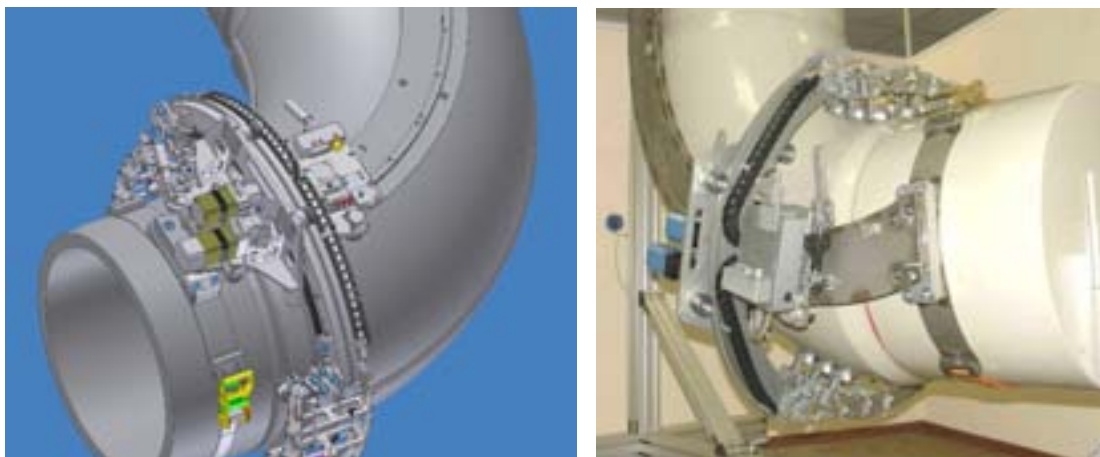
Fig. 7. Specialized scanner SC.590. On the right – the full-size pipe elbow stand simulator of the main circulating pipeline of reactor VVER-440.
