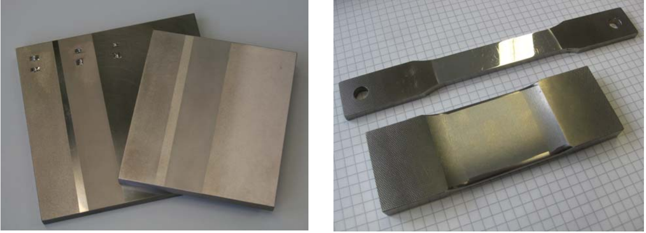
FIGURE 3. left picture: shot peened specimens made of IN718 (upper) and Ti6Al4V (below); right picture: tensile test specimen for measuring SAW parallel and perpendicular to stress direction
