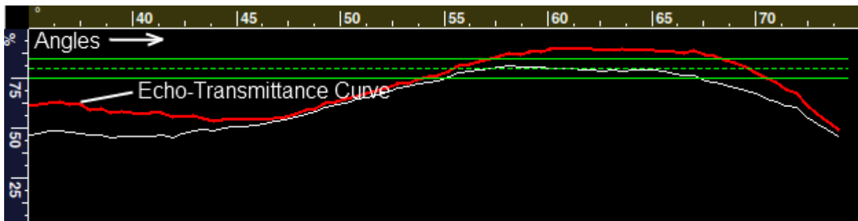
Figure 2: Example of echo-transmittance curve on IIW radius at 100mm with an unfocused array transducer
