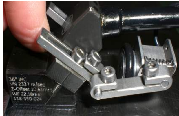
Fig. 4: Phased array probe with position en-
