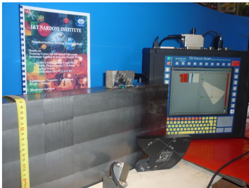
Fig.2 Test block with embedded planar slits of 5x5x0,2 mm distributed along the vertical axis as indicated in fig. 5 (block N°2). Equipment used for the research has been AGR TD- FOCUS SCAN.
