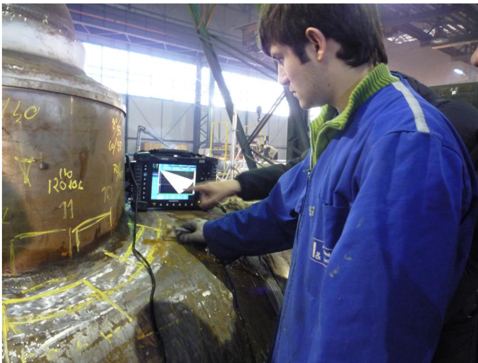
Fig.18 Technician during Phased Array examination of a nozzle relative to fig. 16 with lack of fusion
