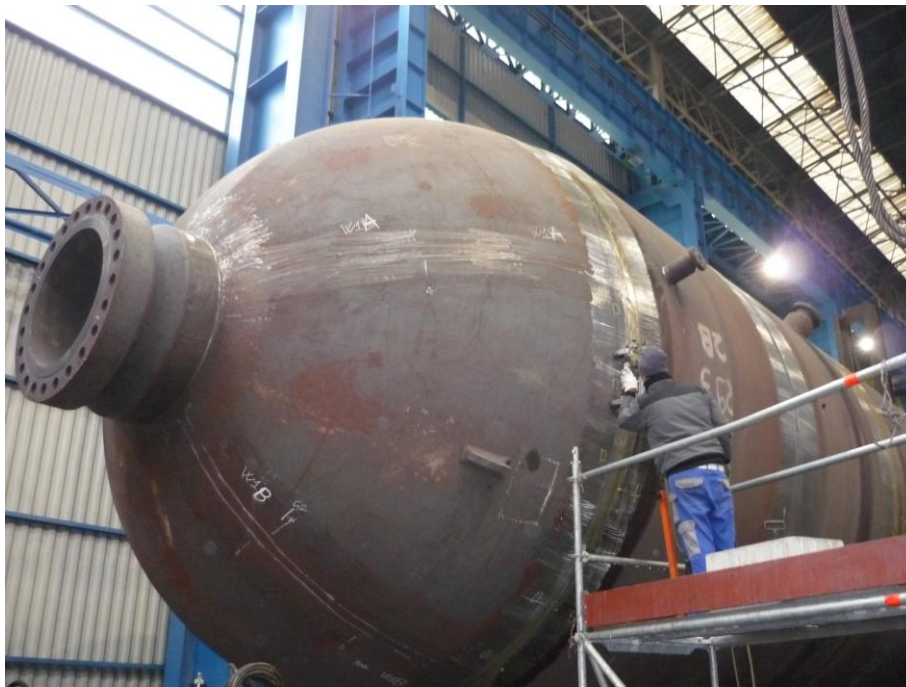
Fig.1 Pressure vessel reactor during ultrasonic examination using computerized technique (TOFD – PHASED ARRAY – C-B SCAN).
