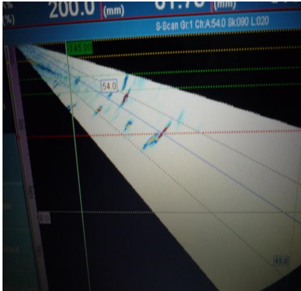
Fig.17 S/B scan presentation of sectorial scan, on 120 mm thickness weld, of lack of fusion type defect.
