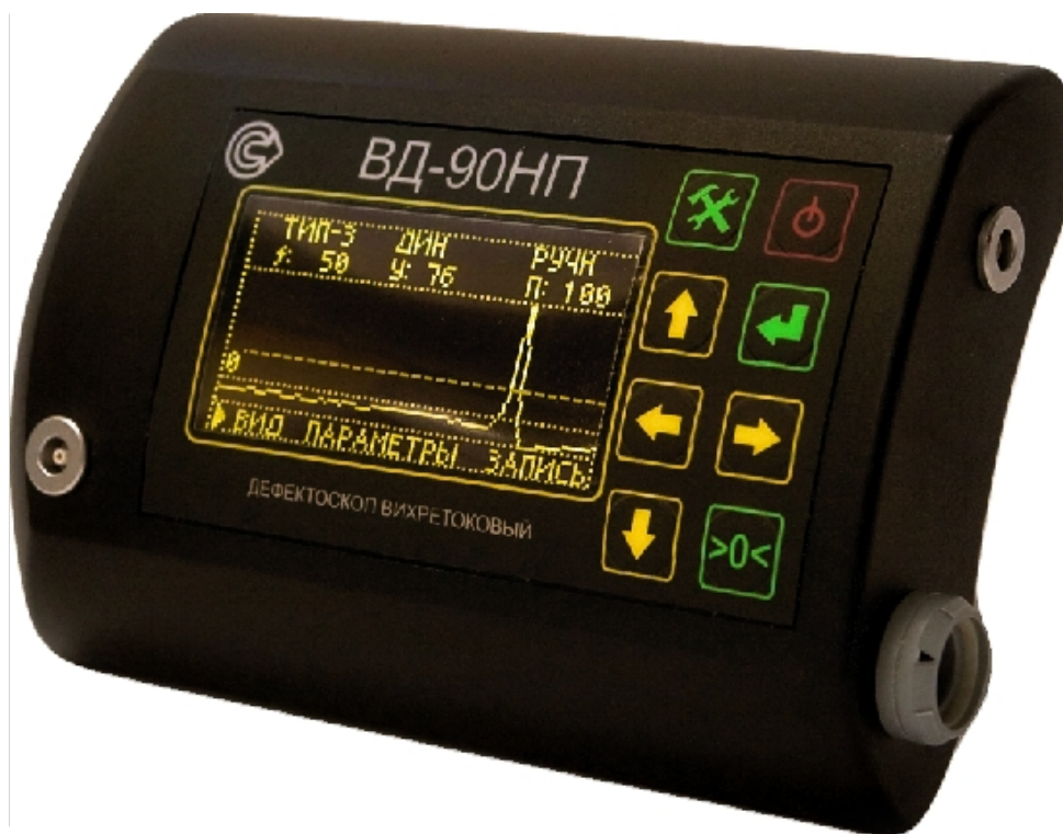
Figure 1. VD-90NP eddy current flaw detector. General view.
