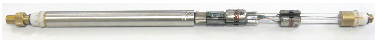
USB connector and centering Housing of 4-channel EC electronics 4 parallel working arrays centering
