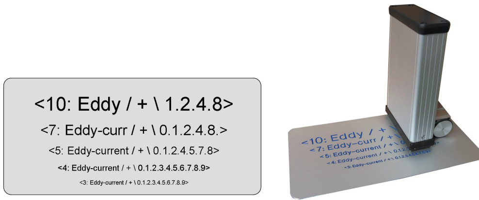
Fig. 6: Engraved aluminium sheet as reference (left). The first number in the line indicates the font size in millimetre. Right: array sensor 64 with measuring wheel on the sheet.
