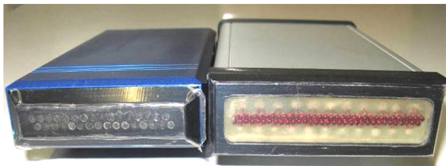
Fig. 5: Left: Array probe 32, 1.5-mm-ferrite rod cores, pitch-catch mode, coil centre distance 3 mm, total track width 45 mm, probe centre distance 1.5 mm, right: Array probe 64, 1.05-mm-ferrite rod cores, pitch-catch mode, coil centre distance 2 mm, total track width 61 mm, probe centre distance ca. 1 mm
