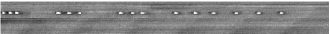
Fig. 12: Circumferential C-Scan image of an austenitic steel tube of 21 mm inner diameter with standard calibration defects of different distance. The scan consists of 36 sensor tracks, scan length about 600 mm.
