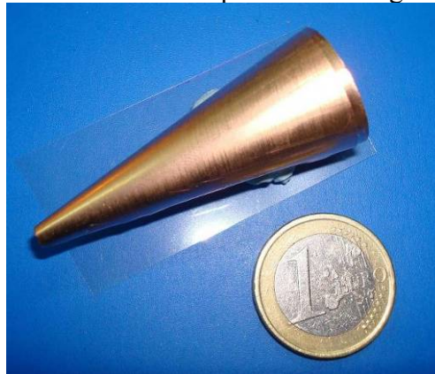
Figure 3. Conical Swiss roll made from LONGLITE TM 200
