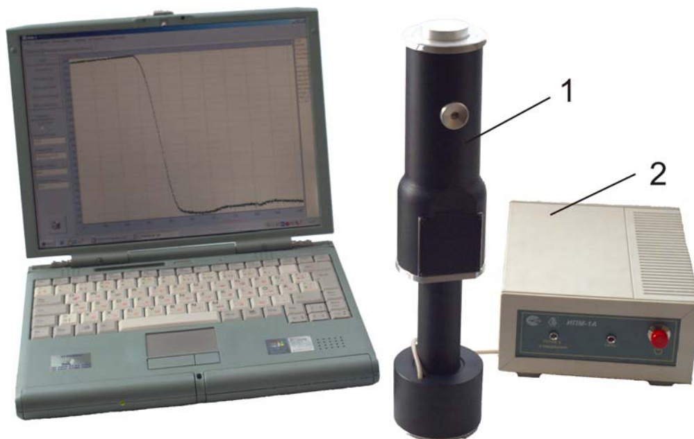
Fig. 2. Installation IPM-1A: 1 – impact gauge, 2 – electronic module
