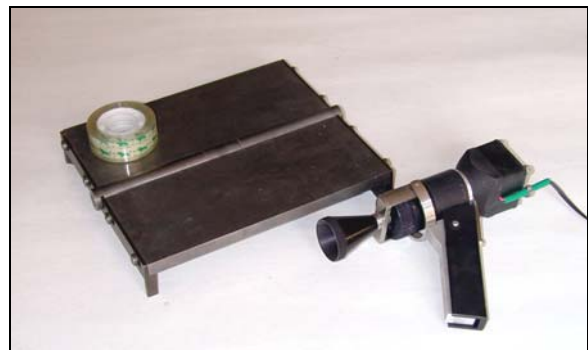
Fig. 2 Production accessories for MPK (a weld seam simulator, a magnetic particle sprayer and a scotch tape for recording)
