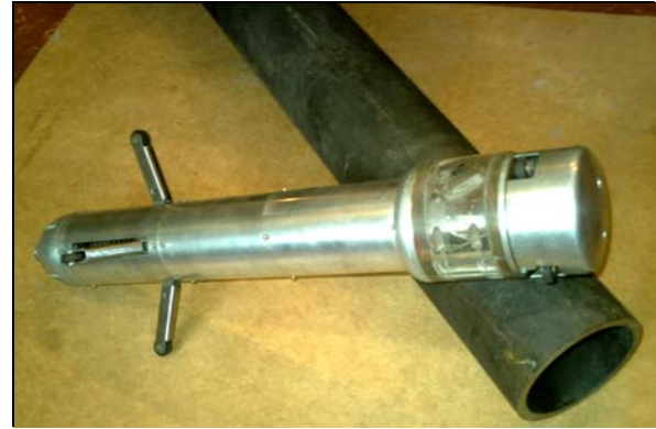
Fig. 4 Self-moving detector with ferroprobe transducer to inspect internal surfaces of industrial pipelines
