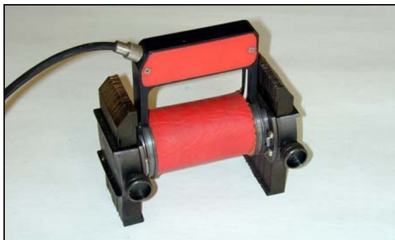
Fig. 1 Magnetizing device MDS -3 conforming the inspected surface
