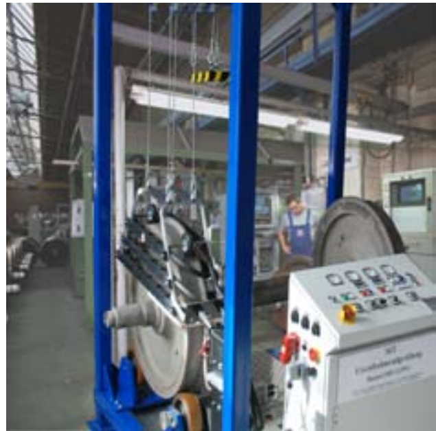
Picture 7. MT Device for railway wheels testing at a train overhaul plant
