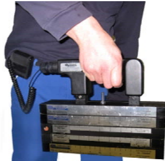
Picture 9. UM-10 lifting test with TB10 test blocks
