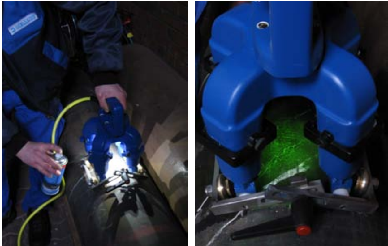
Picture 6. KMU 8/42 with inductive White (left) and UV (right) LED Light Sources
