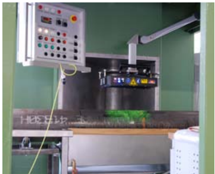
Picture 2. Pipe delivery to magnetizing station (left). Pipe inspection under UV radiation (right)
