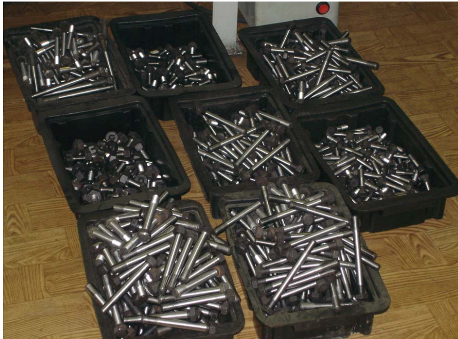
Fig.10 The bolts, tested by the magnetic nondestructive method and returned to production on the Minsk motor plant.
