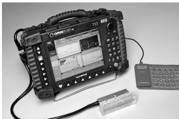
Fig. 5. Ultrasonic phased array inspection
