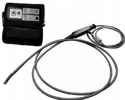
Fig. 1. Flexible ETG endoscope with BOA-20 lighting unit
