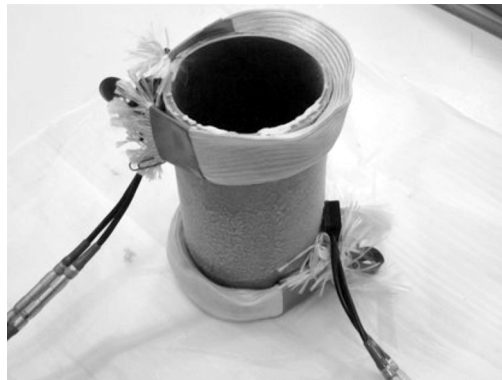
Fig. 1. Low temp. tests on sample pipe
