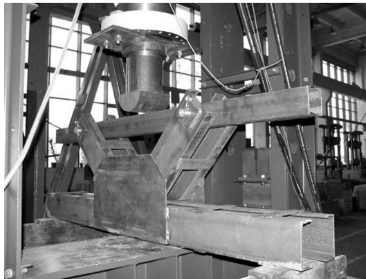
Fig. 1. Full scale steel St3S bridge joint
