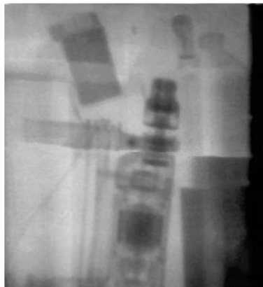
Left – photo of objects layout in a lead box (the near wall is removed to show the content); right – radiographic image obtained with a portable generator of 14 MeV neutrons ING-07 at exposure time 30 min:
