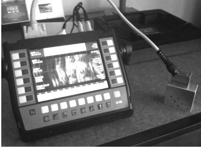
Fig. 2. Material scanning using phased array technology
