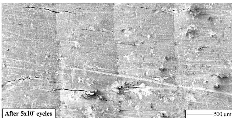
Fig. 1. Effects of fatigue loading in corrosive environment
