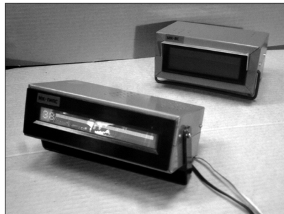
Fig. 7. Indicators capable to display line-by-line results and to subsequently distribute signals to a sorting machine
