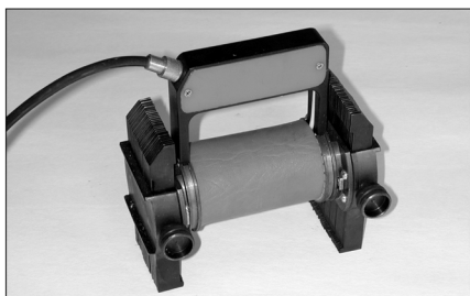
Fig. 1. Magnetizing device MDS -3 conforming the inspected surface
